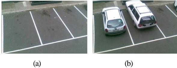
**Fig. 1. (a) A reference image where the parking lot is empty. The same set of filter is applied to the reference image as well as the incoming image stream represented by (b). For images streams where the vehicle colour is light (as in (b)), it is rather easy to obtain a high detection accuracy.**
