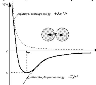
**Figure 9: Van der Waals Potential Energy**
