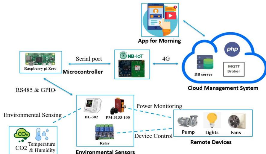
**Figure 3. The architecture of the proposed greenhouse environment monitoring system.**
