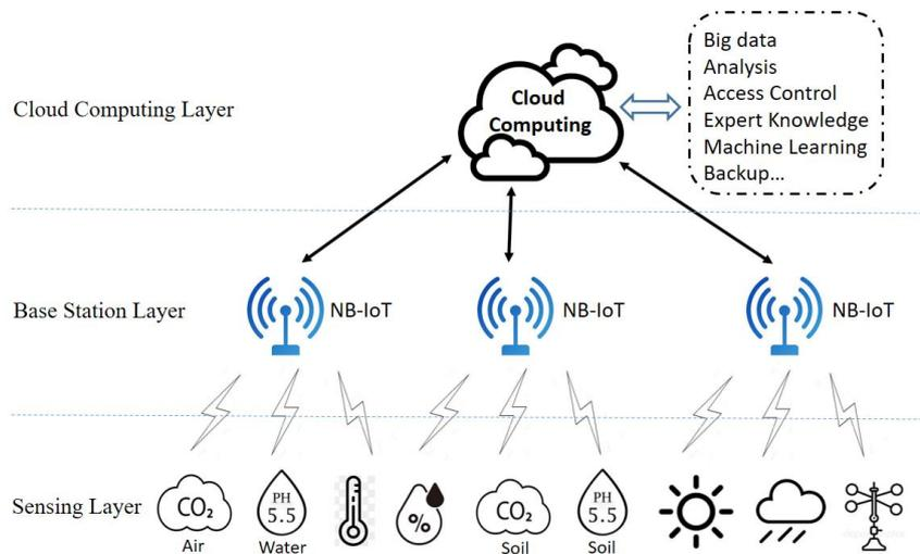
**Figure 1. The architecture for connecting intelligent sensors in smart agriculture.**
