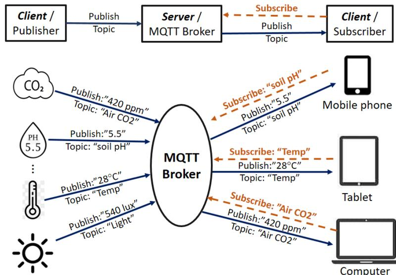
Figure 5. Architecture of publishers and subscribers with sensors and MQTT broker.
