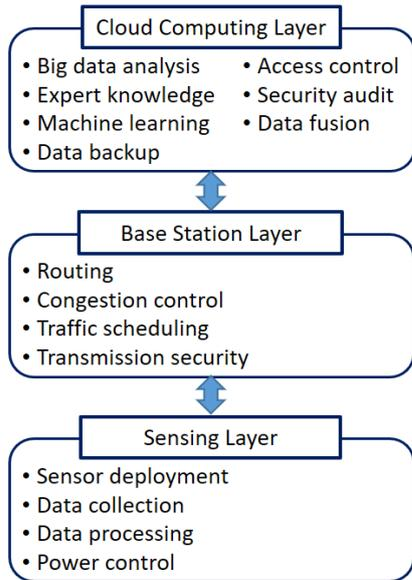
**Figure 2. Main function and design requirements for each layer in the proposed architecture.**
