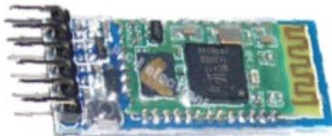
Figure 5. The appearance of the HC-05 module
