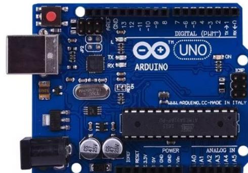
Figure 3. Arduino development board
