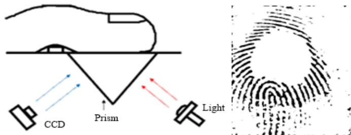
Figure 3. Traditional fingerprint image capture device setup.
