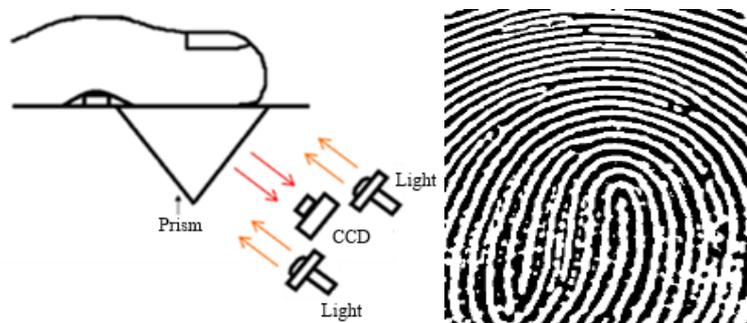
Figure 4. Modified fingerprint image capture device.
