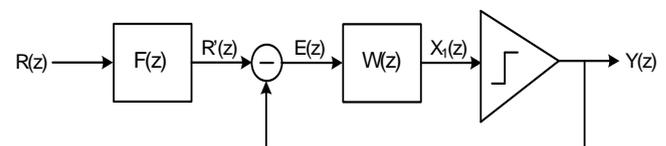
Fig. 3.3 Sigma-Delta Equivalent Model
