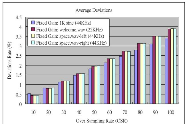
Fig. 4.5 Fixed Gain Case for Average Deviations between Restore Signal and Original Signal
