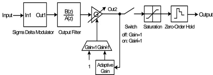
Fig. 3.6 Anti-Noise architecture with an adaptive gain
