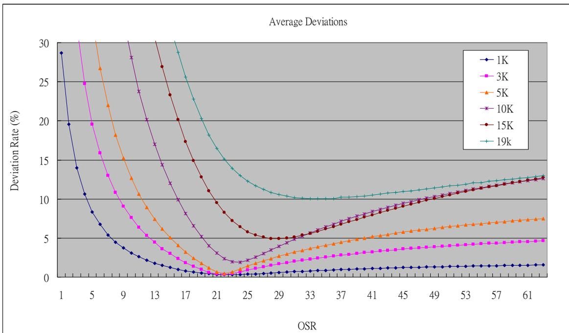
**Fig. 4.9 Relationship between OSR and Average Deviations of signal from 1 KHz to 19 KHz sine wave**
