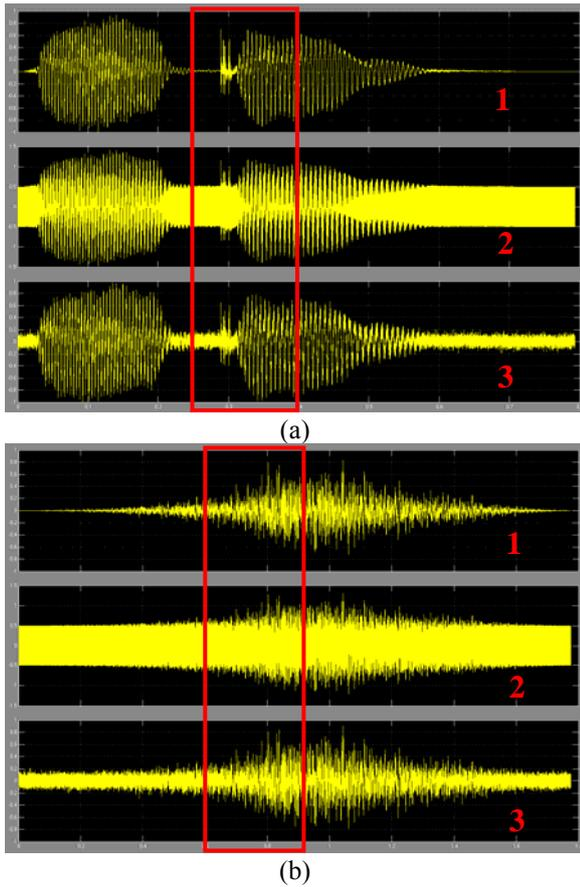
Fig. 4.3 the audio signals “welcome” and “space”, (a)Waveform in Each Stage of welcome.wav, (b) Waveform in Each Stage of space.wav.
