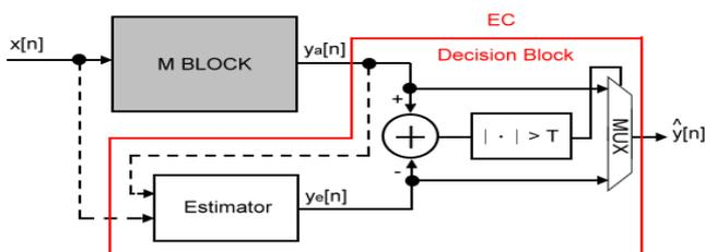
Fig. 2.1 Algorithmic Noise-Tolerance (ANT)
