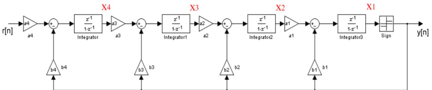
Fig. 3.2 Fourth-Order 1-Bit Sigma-Delta Modulator
