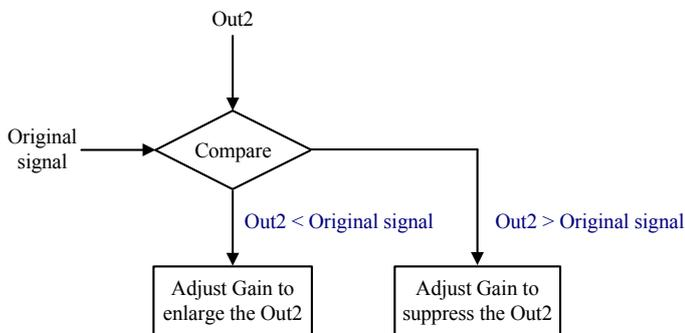
Fig. 3.7 A new self-inverse unit-gain method
