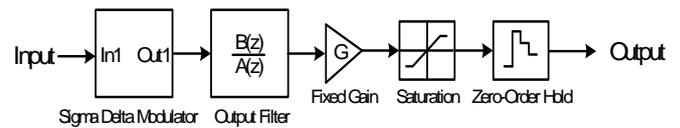
**Fig. 3.5 Anti-Noise System Architecture (Self Noise Tolerance Estimator)**
