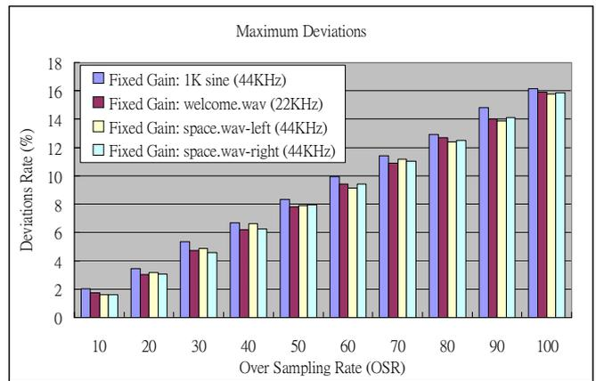
Fig. 4.4 Fixed Gain Case for Maximum Deviations between Restore Signal and Original Signal
