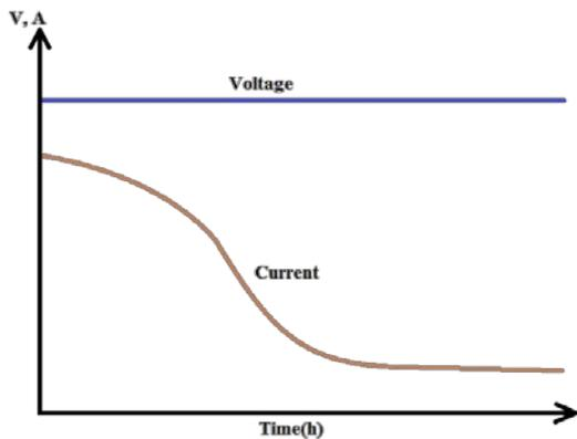
**Fig. 1** Charging curve using CV mode
