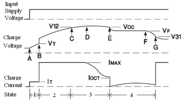
Fig. 7 Four state charge diagram
