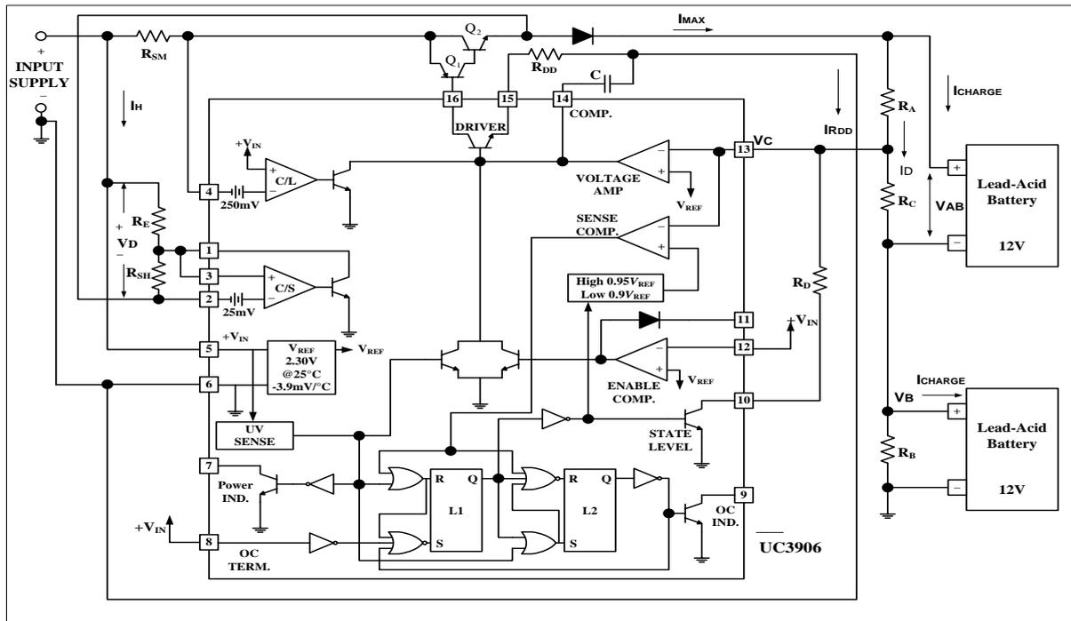
Fig. 8 Hardware of multi-state charge controller
