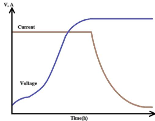
**Fig. 3** Charging curve using CV-CC mode
