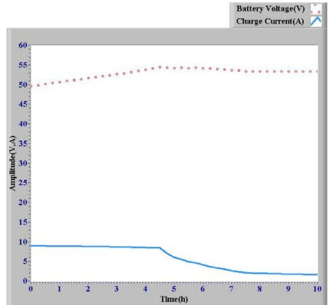
Fig. 15. Charging curves using  $I_{MAX} = 9A$ , Case 7:
