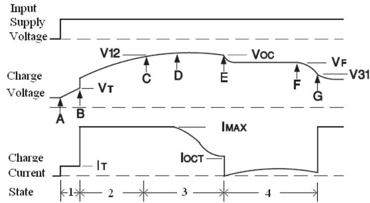
Fig. 7 Four state charge diagram
