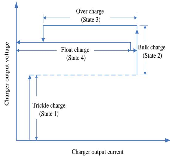
**Fig. 6 Four state charge diagram**
