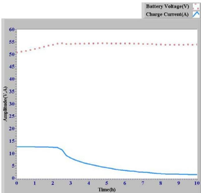
Fig. 17. Charging curves using  $I_{MAX} = 13A$ , Case 9:
