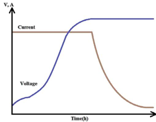
**Fig. 3 Charging curve using CV-CC mode**
