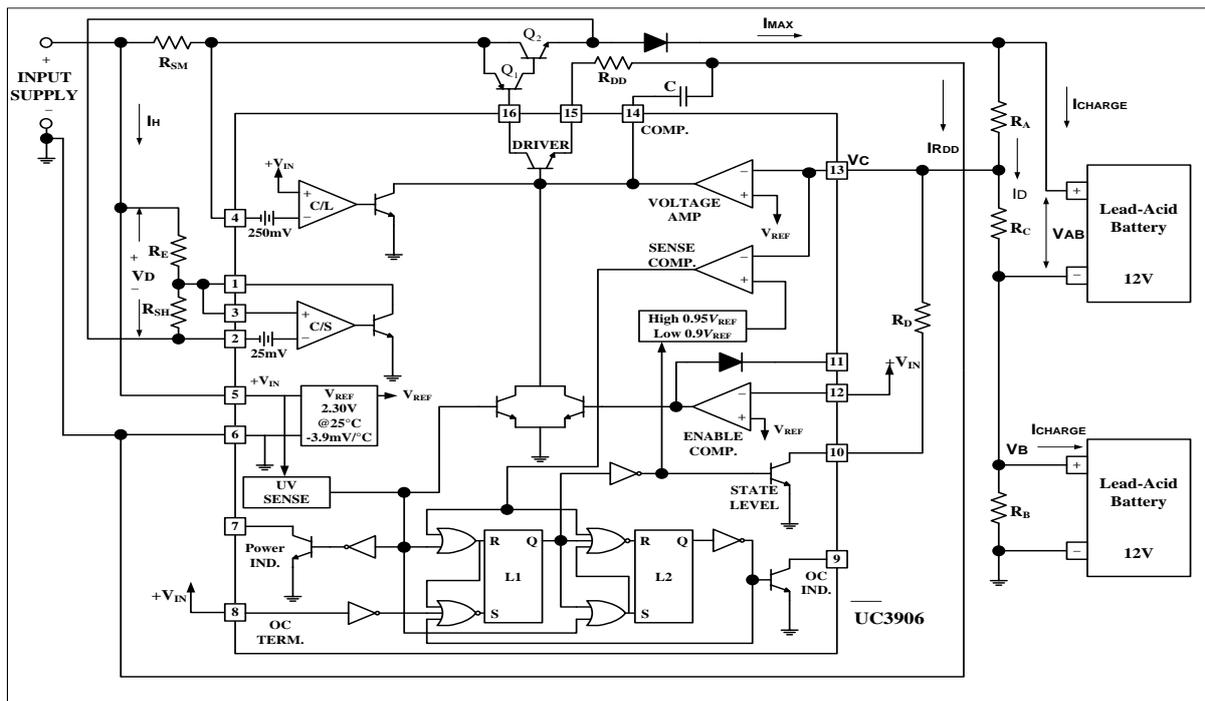
Fig. 8 Hardware of multi-state charge controller
