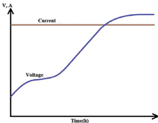
**Fig. 2** Charging curve using CC mode
