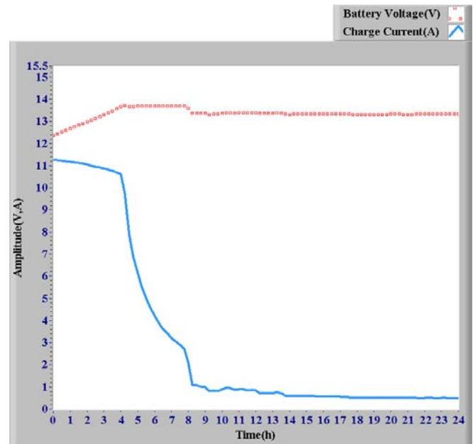
Fig. 11. Charging curves using  $I_{MAX} = 11A$ , Case 3:
