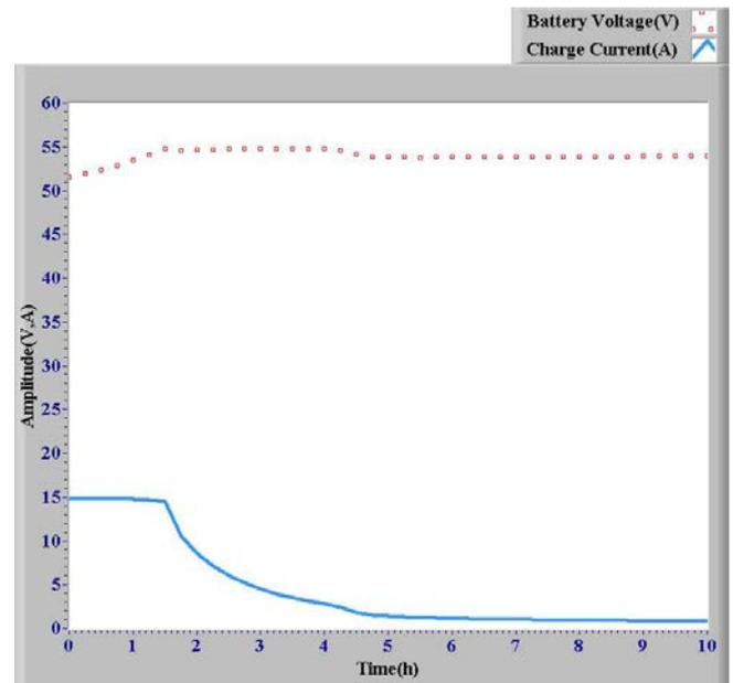
Fig. 18. Charging curves using  $I_{MAX} = 15A$ , Case 10:
