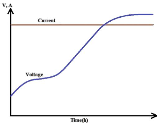
**Fig. 2 Charging curve using CC mode**
