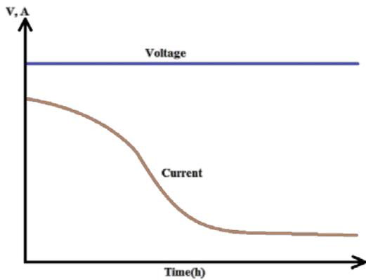
**Fig. 1 Charging curve using CV mode**
