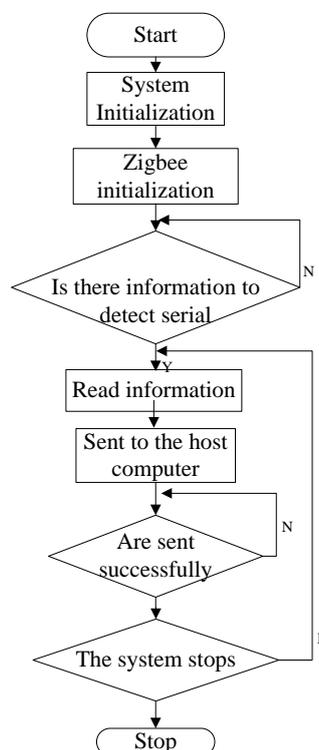
Figure 4: Zigbee detection system flowchart
