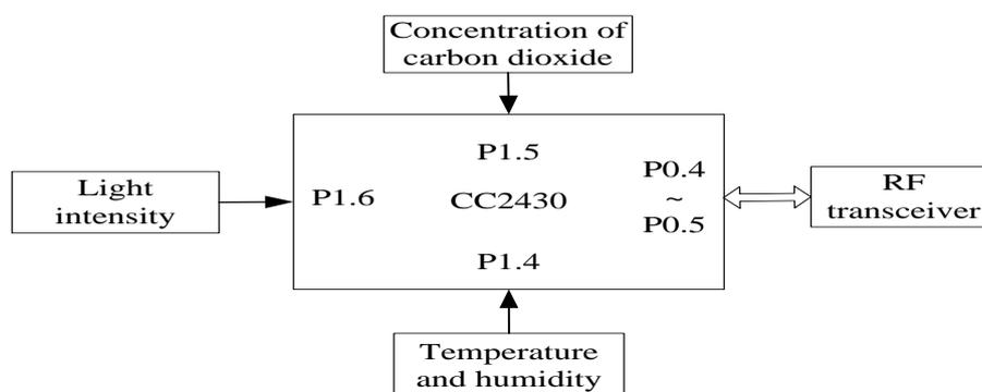
**Figure 2: a block diagram of detection system**
