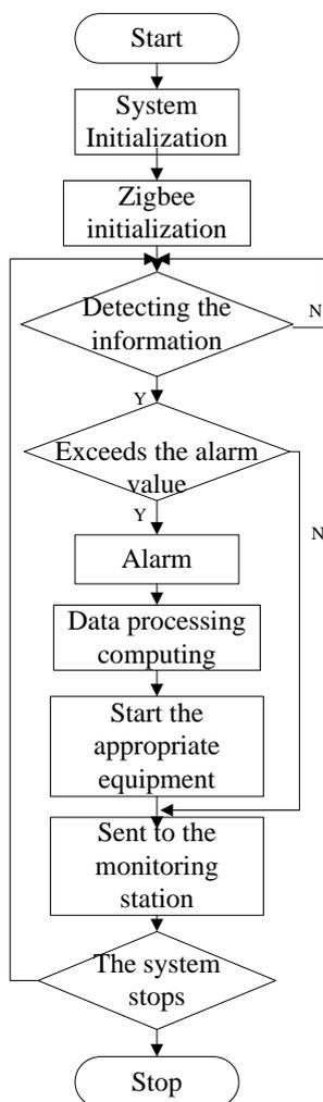
Figure 5: Program flow monitoring system
