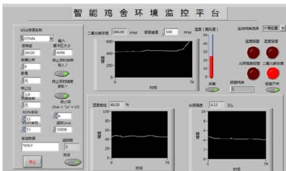
Figure 8:PC interface displays the carbon dioxide concentration in excess of the alarm
