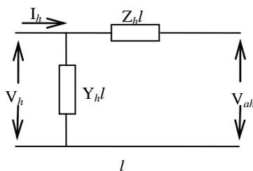
Figure 2: line equivalent circuit
