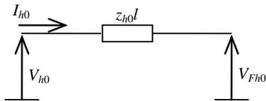
Figure 7: zero-sequence equivalent circuit
