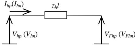
Figure 6: positive- and negative-sequence equivalent circuits
