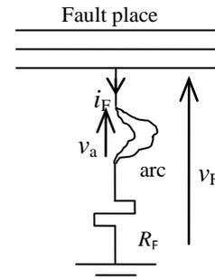
Figure 3: Fault model given in time domain
