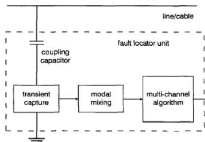
**Figure 9: Block diagram of fault locator unit**
