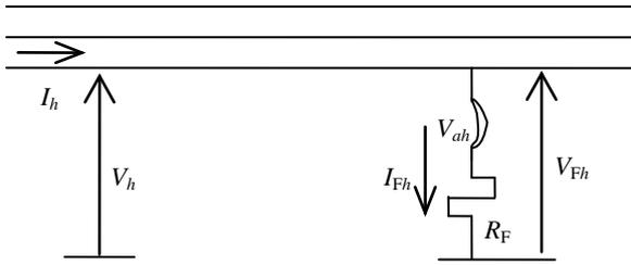
Figure 5: Single-phase-to-ground arcing fault
