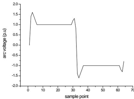
Figure 1: arc voltage wave shape
