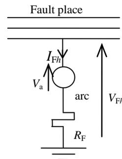
Figure 4: Fault model given in spectral domain
