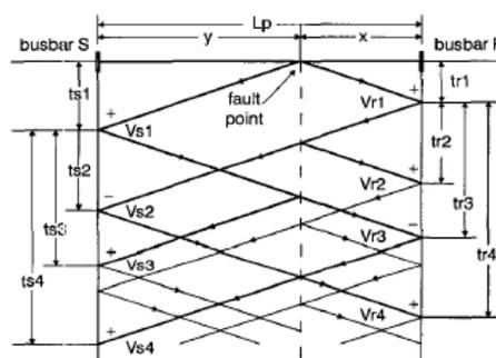
**Figure 8: Lattice diagram for single-phase loss-free overhead line**
