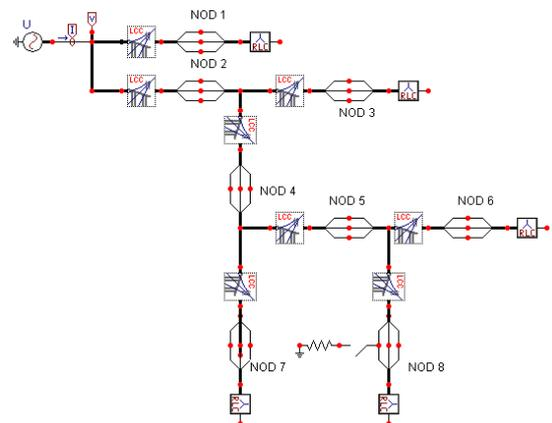
Figure 9: simulation model of distribution network
