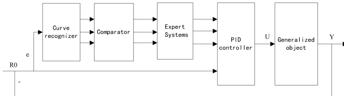
Figure 1: expert-type self-tuning PID controllers automated system structure diagram
