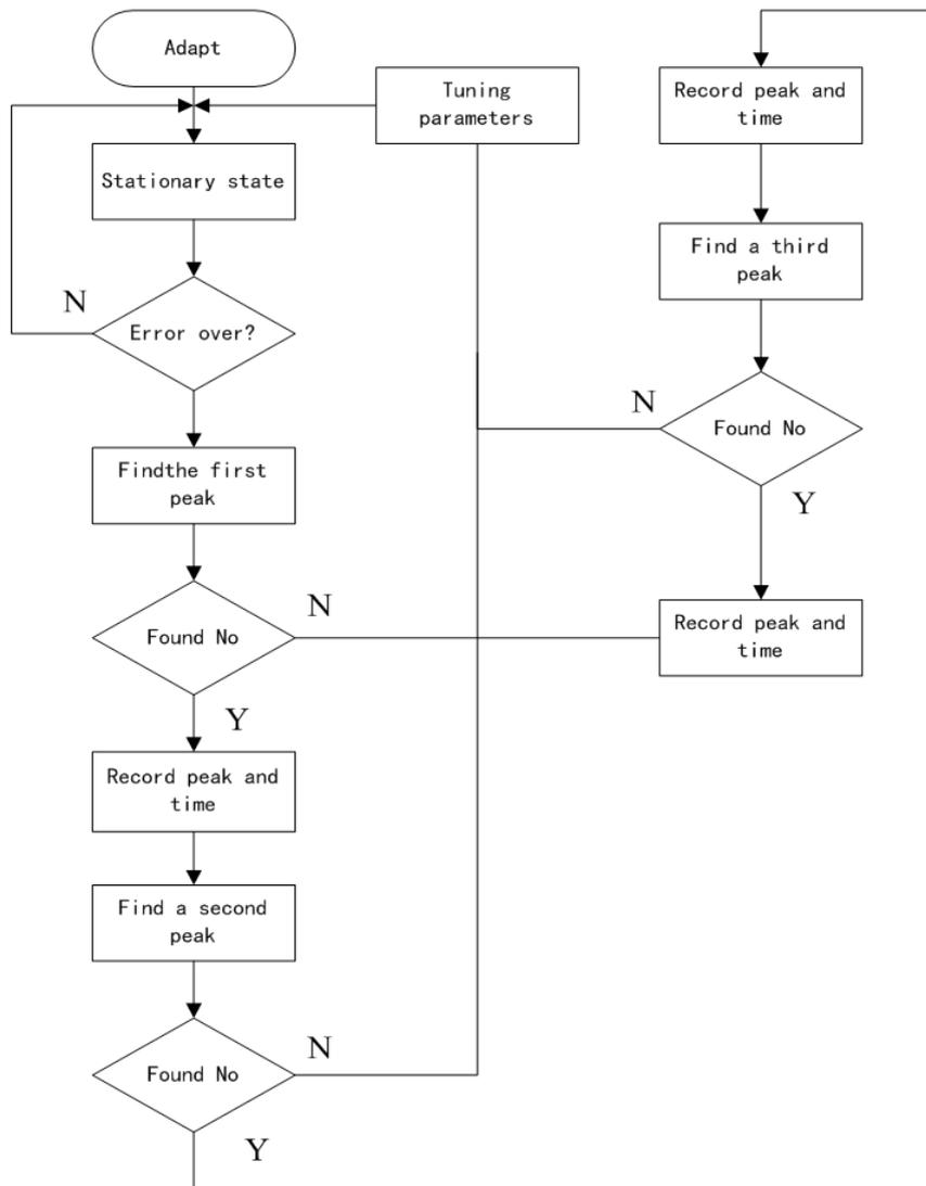
Figure 3: Automatic identification block diagram
