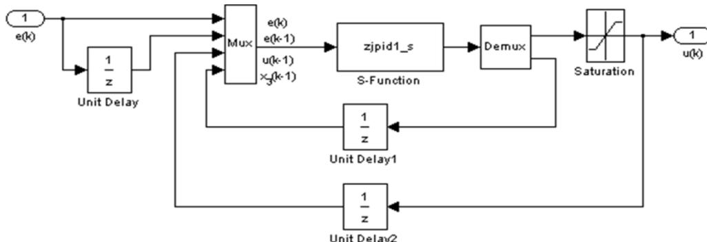
Figure 5: expert system PID controller
