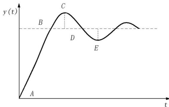
**Figure 2: A typical step response of second-order system**
