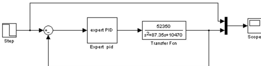
Figure 4: PID controller simulation expert system structure diagram
