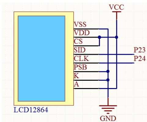
Figure 5: SCM and 12864 connection diagram
