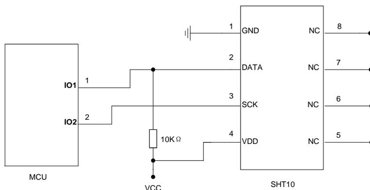
Figure 3: microprocessor hardware connection diagram with SHT10
