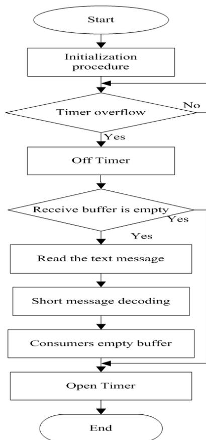
Figure 10: Receiving SMS program flow
