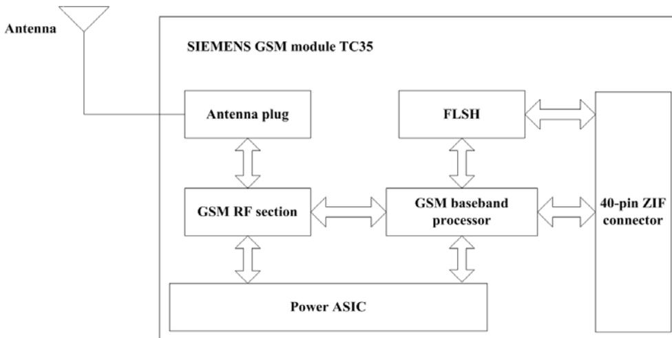
Figure 2: TC35i module structure diagram
