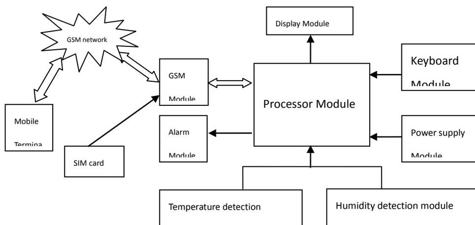
**Figure 1: The overall block diagram of the system**
