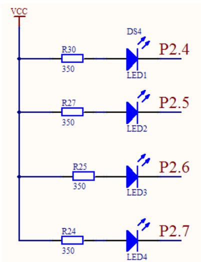
Figure 7: LED alarm circuit
