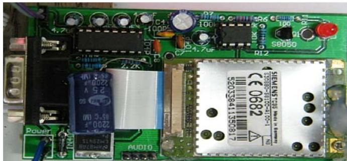
Figure 11: GSM module physical map
