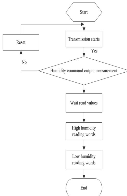
Figure 8: Program flow measuring temperature and humidity
