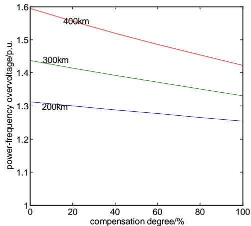
Figure 7: The influence of compensation degree to power-frequency overvoltage when HV shunt reactor at sending end of the line
