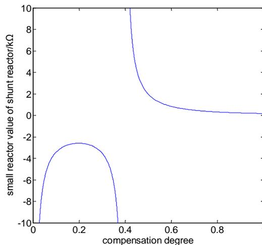
Figure 12: The relationship between small reactor value of shunt reactor and compensation degree
