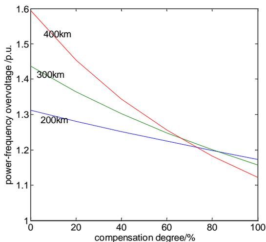
Figure 6: The influence of compensation degree to power-frequency overvoltage when HV shunt reactor at receiving end of the line
