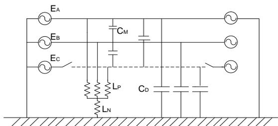
Figure 10: Schematic diagram of open-phase operation
