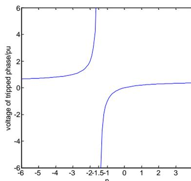
Figure14: The relationship between voltage of tripped phase and n
