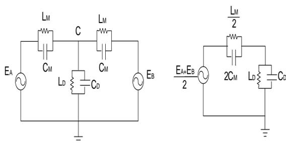
(a) The equivalent figure of open-phase operation
