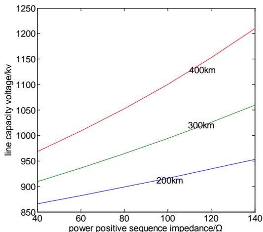
**Figure 3: The influence of the power positive sequence impedance to line capacity voltage rise**
