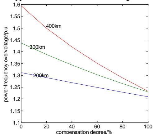
(a) power-frequency overvoltage when m end three-phase tripping
