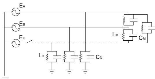
Figure 11: The equivalent figure of open-phase operation with high voltage shunt reactor
