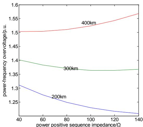
**Figure 4: The influence of the power positive sequence impedance to power-frequency overvoltage**
