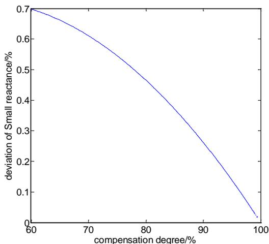
**Figure 15: The relationship between compensation degree and deviation of Small reactance**
