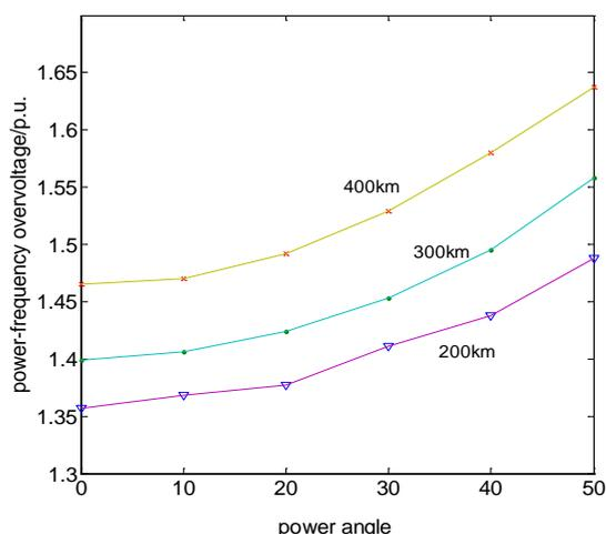
Figure 1: The influence of the power angle to power-frequency overvoltage
