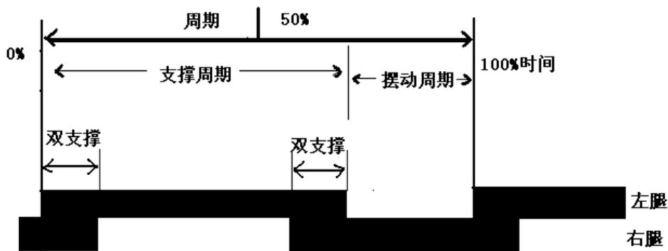
Figure 6: gait cycle diagram
