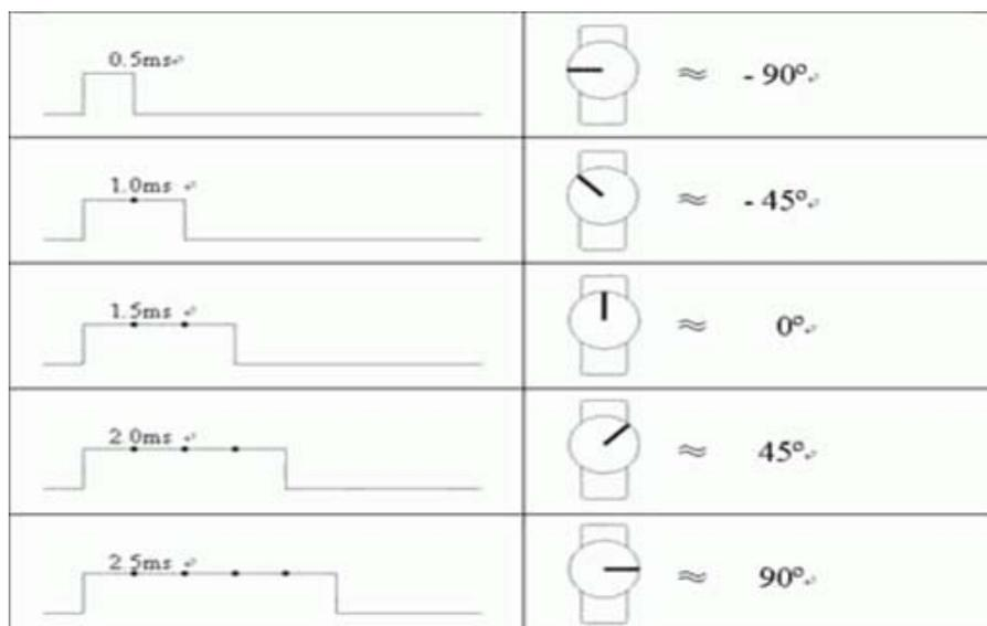
Figure 5: Servo output pulse width corresponding to the position location map
