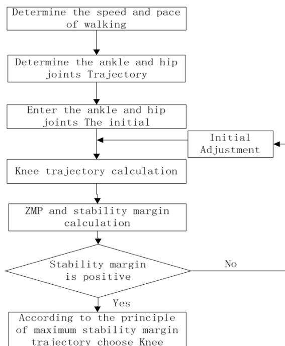
Figure 7: Biped robot gait planning flowchart
