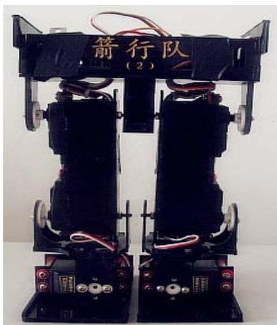
**Figure 1: biped robot front view**
