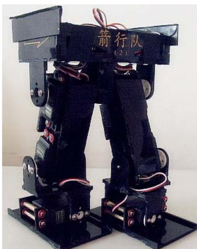
**Figure 2: biped robot side view**
