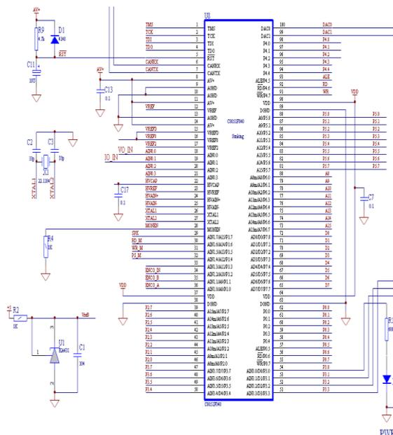
Figure 4: C8051F040 peripheral circuit
