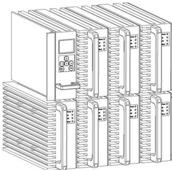
**Figure 14: Structure diagram of multi- power modules with control units**
