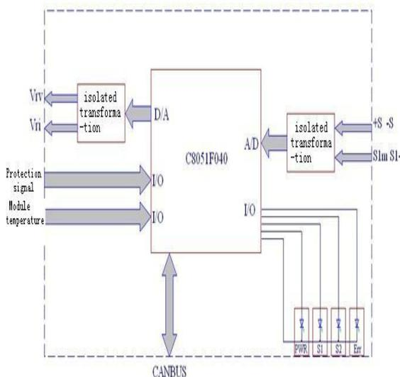
Figure 3: Digital control circuit diagram
