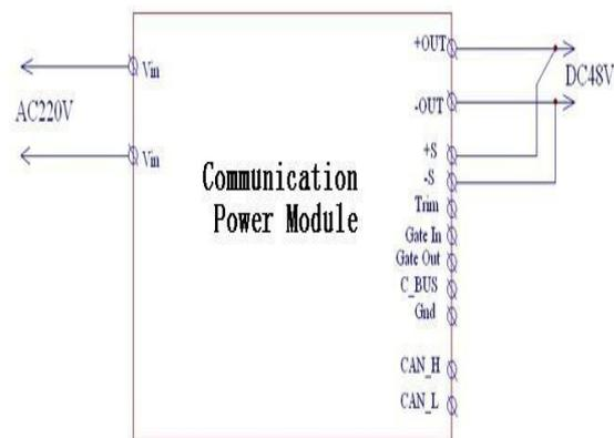
Figure 9: Diagram of single module usage
