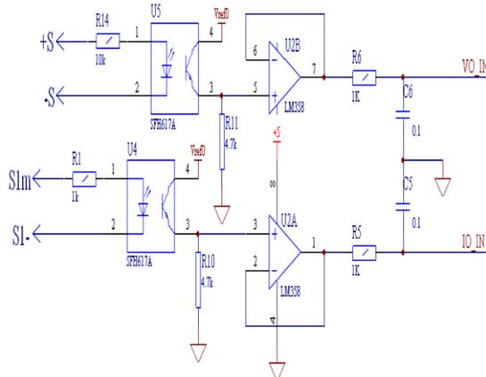
Figure 5: Input circuit of ADC
