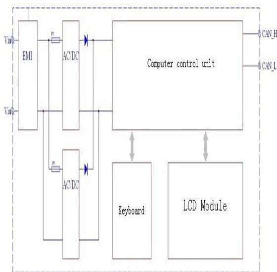
Figure 7: Block diagram of central control unit
