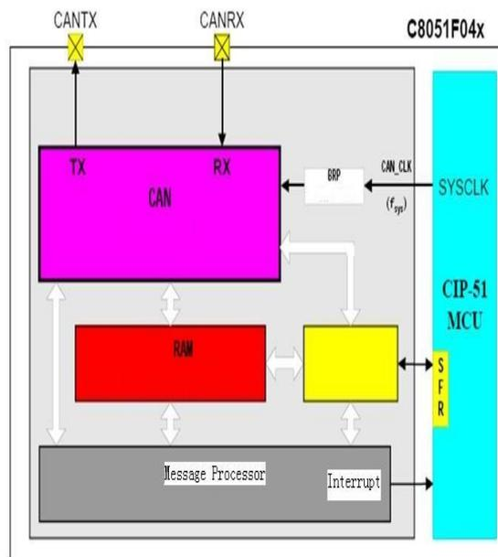
Figure 1: Block diagram of the CAN controller
