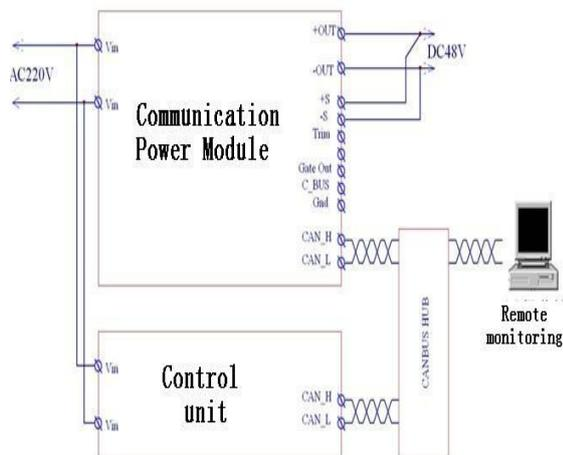
Figure 10: Diagram of single module with control unit
