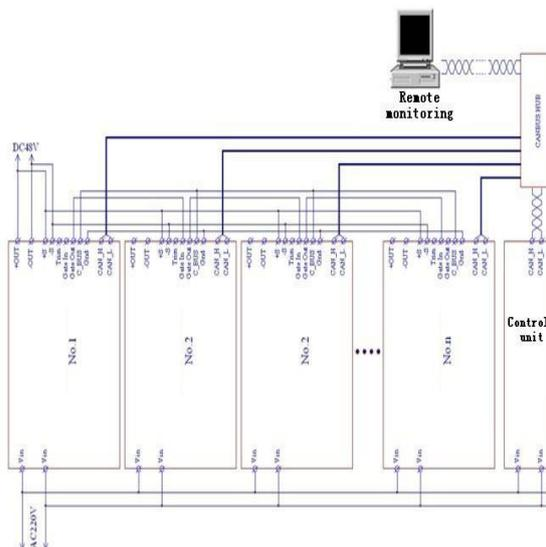
Figure 13: Diagram of multi- power module with control unit
