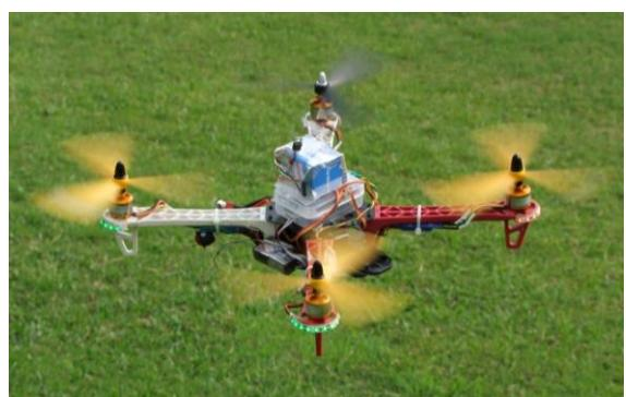
**Figure 9:** The experimental quad-rotor UAV.
