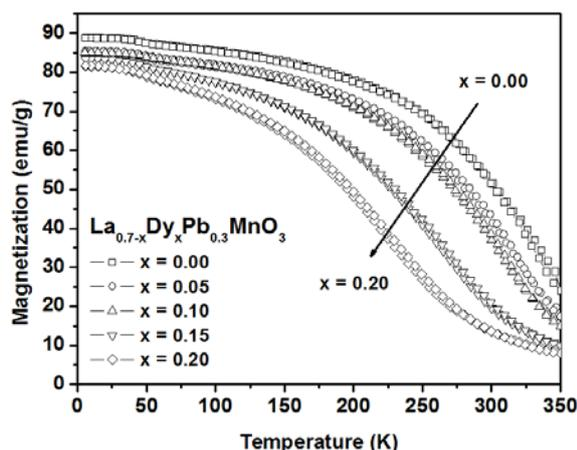
**Figure 3: Temperature dependence magnetization measured at an applied field of 5 teslas for all polycrystalline  $\text{La}_{0.7-x}\text{Dy}_x\text{Pb}_{0.3}\text{MnO}_3$  perovskites.**
