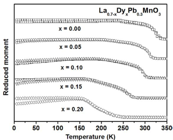
Figure 2: Temperature dependence magnetization measured at a low field of 100 Oe for all polycrystalline  $\text{La}_{0.7-x}\text{Dy}_x\text{Pb}_{0.3}\text{MnO}_3$  perovskites.
