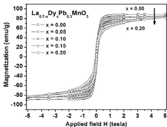
**Figure 4: Magnetic hysteresis curves for all polycrystalline  $\text{La}_{0.7-x}\text{Dy}_x\text{Pb}_{0.3}\text{MnO}_3$  perovskites.**
