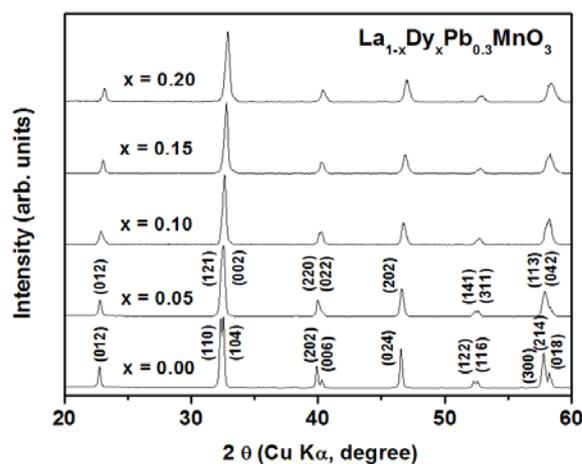
Figure 1: X-ray diffraction spectra for all polycrystalline  $\text{La}_{0.7-x}\text{Dy}_x\text{Pb}_{0.3}\text{MnO}_3$  perovskites.
