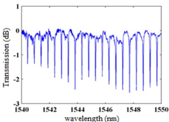
**Figure 8: Transmission spectra of the MKR with knot length of 6 mm.**
