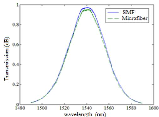
**Figure 3: The optical transmission spectra of the fiber before and after being tapered.**
