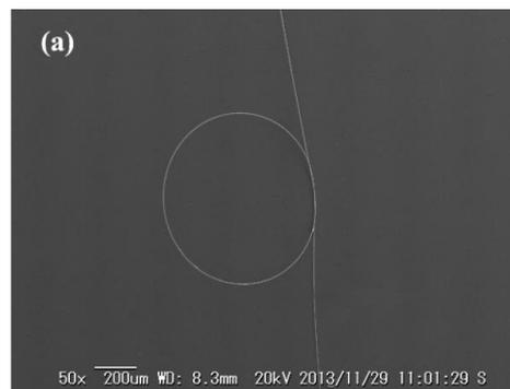
**Figure 4: SEM of the fabricated MKR.**
