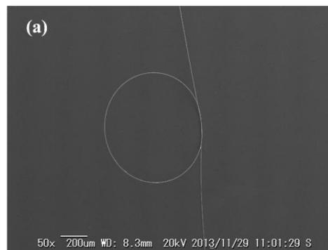
**Figure 4: SEM of the fabricated MKR.**
