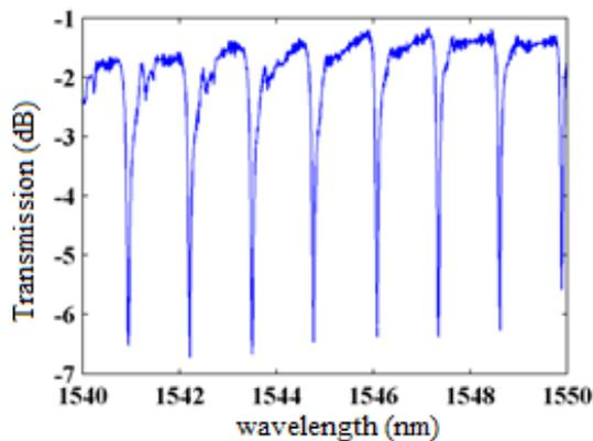
**Figure 7: Transmission spectra of the MKR with knot length of 2.5 mm.**
