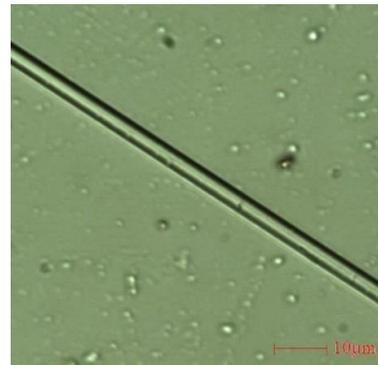
**Figure 2: Microscope image of the fabricated microfiber**
