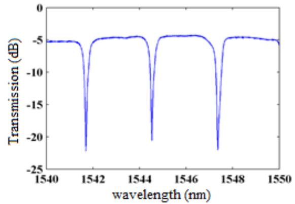
Figure 5: Transmission spectra of the MKR with knot length of 1 mm.
