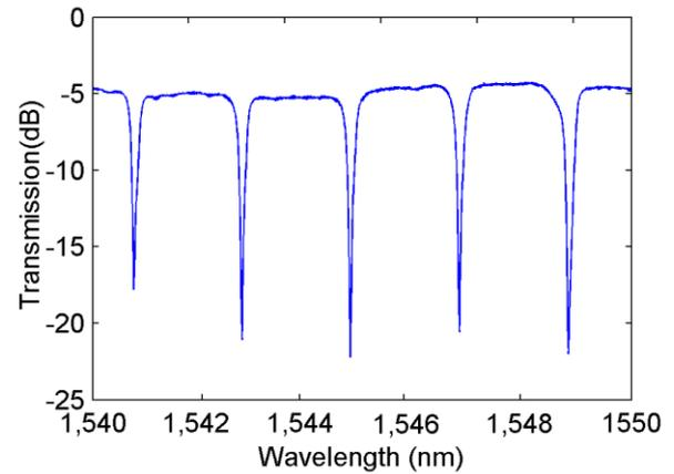
Figure 6: Transmission spectra of the MKR with knot length of 1.8 mm
