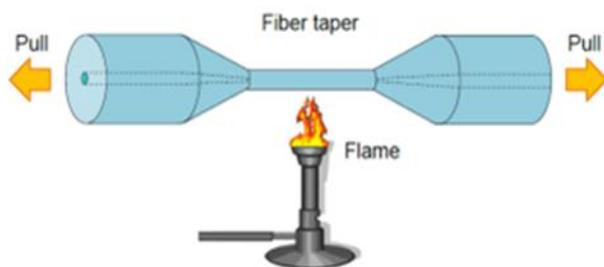
**Figure 1: Schematic diagram of the flame brushing technique**
