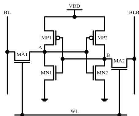
**Figure 1: Circuit diagram of conventional 6T SRAM cell.**
