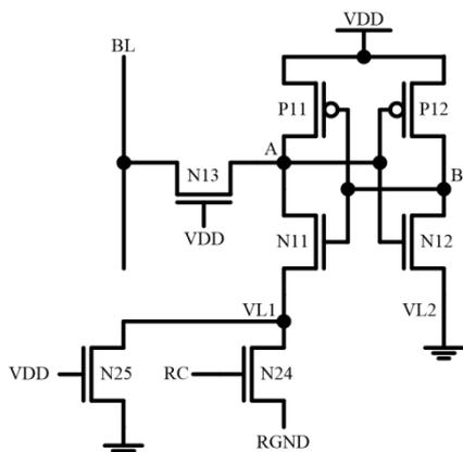
Figure 6: Simplified circuit diagram during the read operation.
