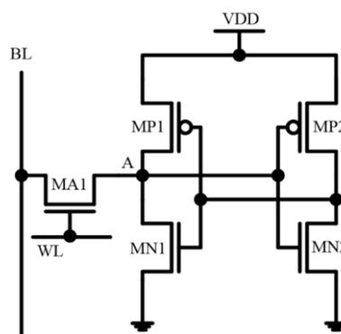
**Figure 2: Circuit diagram of conventional 5T SRAM cell.**
