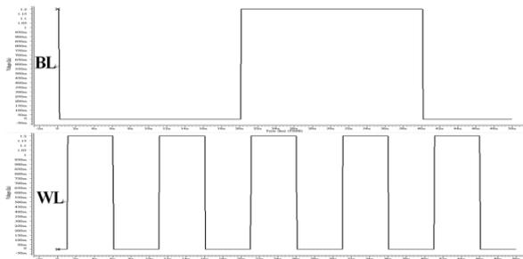
Figure 9: Timing diagram to perform a write operation.
