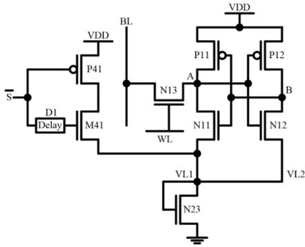
Figure 8: Simplified circuit diagram during the standby operation.
