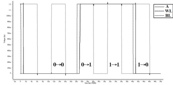
Figure 10: Transient analysis waveforms of writing a data value to the proposed 5T SRAM cell
