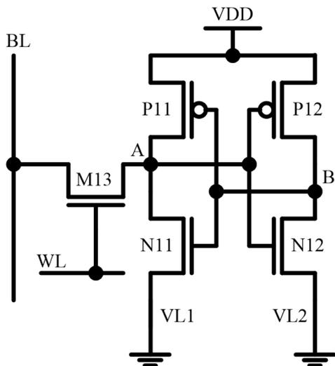
Figure 5: Simplified circuit diagram during the write operation.
