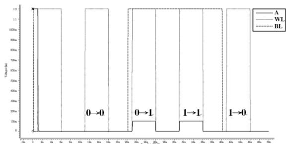
**Figure 3: Transient waveforms of writing a data to the conventional 5T SRAM cell.**
