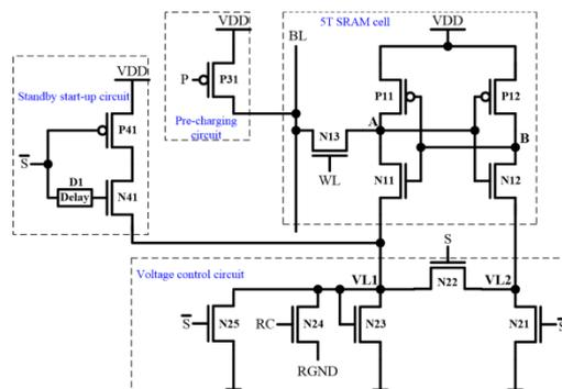
**Figure 4: Circuit diagram of the proposed 5T SRAM cell.**
