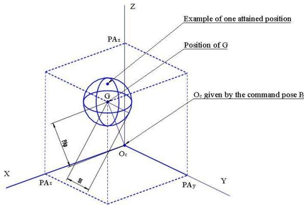
Figure 5: Pose accuracy and pose repeatability
