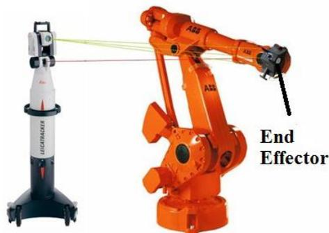
**Figure 1: Laser tracker with tested Robot**
