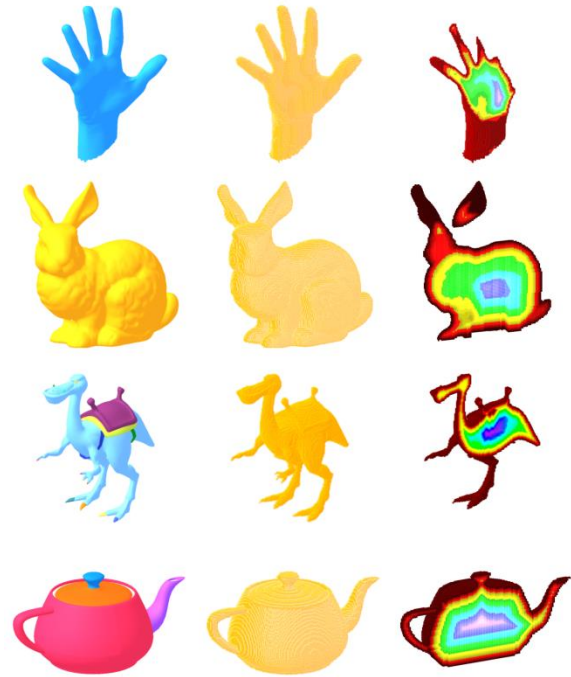
Figure 7: The results obtained from our adaptive voxelization method for the Hand, Bunny, Dinopet, and Teapot meshes: left, the input mesh; middle, the voxel set; right, a sliced-view with coloured distance map.
