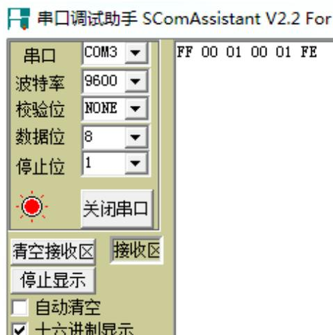
Figure 12: Command received for moving forward
