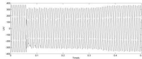
Figure 11: Original waveform of voltage sag caused by common action
