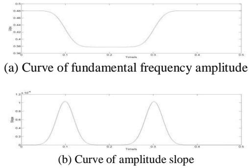
Figure 13: Line short circuit fault
