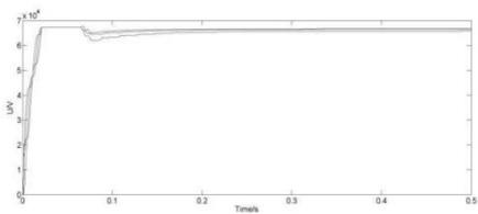
**Figure 6: RMS of voltage sag caused by transform energizing**
