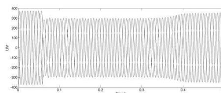
Figure 3: Original signal of voltage sags caused by an induction motor
