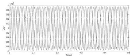
**Figure 5: Original waveform of voltage sags caused by transform energizing**
