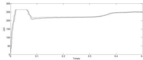
Figure 12: Effective value of voltage sag caused by common action
