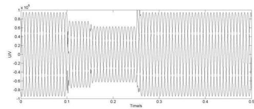
**Figure 7: Original waveform of voltage sag caused by multiple lines short circuit fault**
