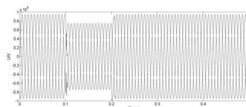
Figure 1: Original signal of voltage sag caused by short circuit faults
