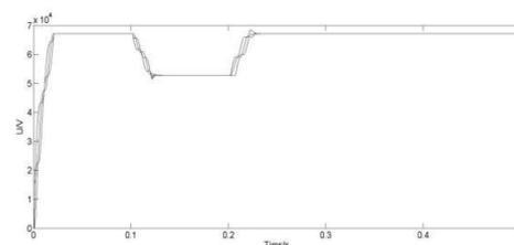
Figure 2: RMS of voltage sag caused by short circuit fault
