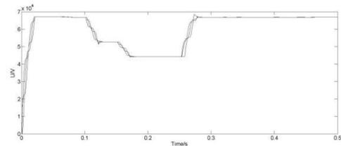
**Figure 8: Effective value of voltage sag caused by multiple lines short circuit fault**
