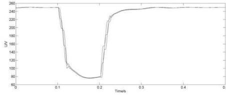
Figure 10: Effective value of voltage sag caused by restarting of induction motor
