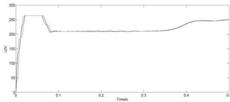
**Figure 4: RMS of voltage sags caused by an induction motor**
