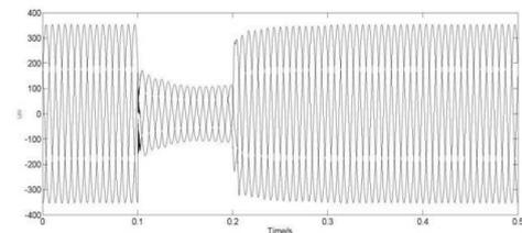
**Figure 9: Original waveform by Induction motor restart induced voltage drop**
