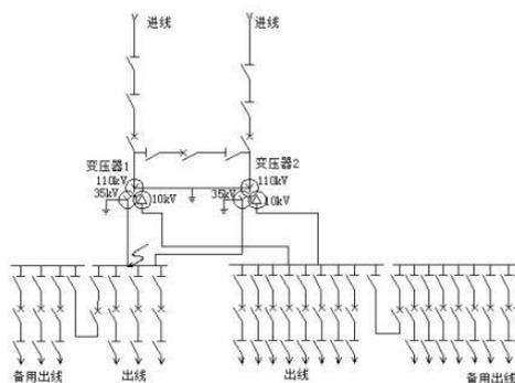
Figure 3: Schematic diagram of 35kV side short-circuit in Substation
