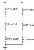
Figure 6: Equivalent circuit of 10kV side short-circuit in Substation
