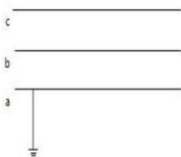
**Figure 7: Schematic diagram of single phase grounding short-circuit**
