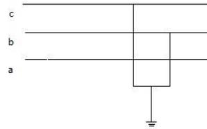
**Figure 11: Schematic diagram of two phase earth fault**
