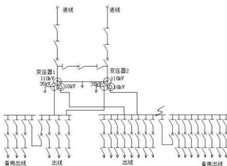
Figure 5: Schematic diagram of 10kV side short-circuit in Substation
