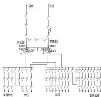
Figure 1: Schematic diagram of 110kV side short-circuit in Substation
