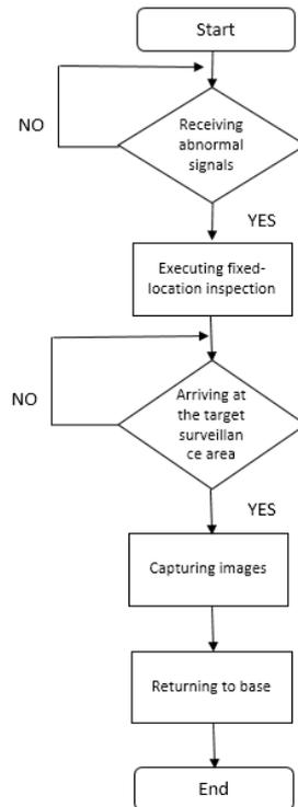
**Figure 3.5: Fixed-location Inspection Process (UAV activated when abnormal signals are received or residents have reported incidents)**
