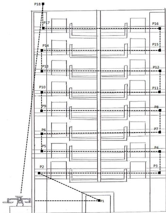
**Figure 3.4: Fixed-location Patrol's Schematic Diagram (P1-P26 are patrol points)**
