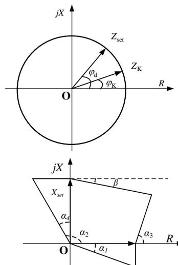
Figure 2: Circle and polygon operating characteristics of distance protection
