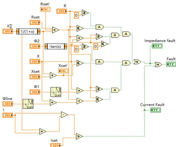
Figure 8: Block diagram of fault judgment module
