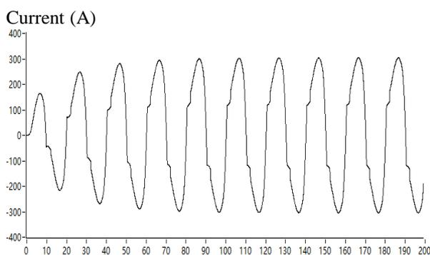
Figure 11: Current waveform of the AC side
