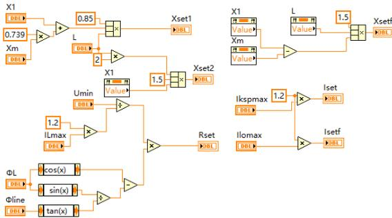
Figure 7: Block diagram of setting module
