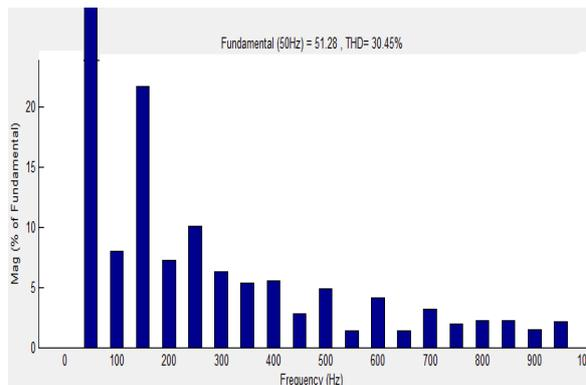
Figure 13: Harmonic analysis of AC side current
