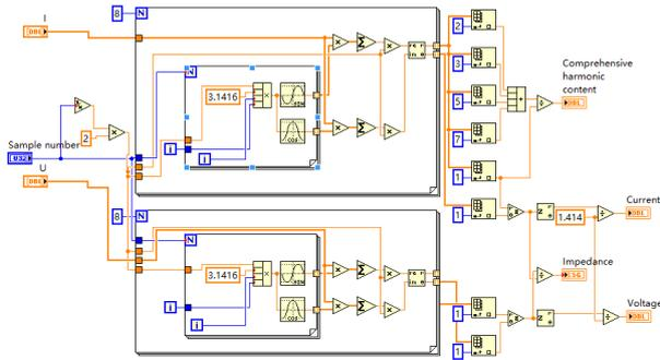
Figure 6: Block diagram of harmonic analysis module
