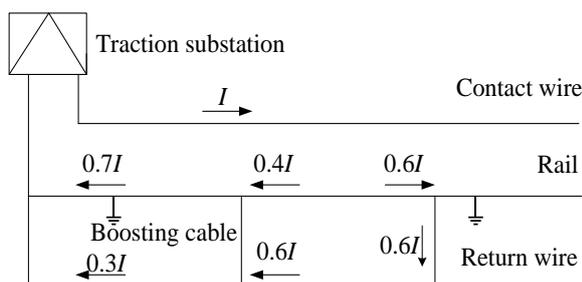
Figure 1: Diagram of DN power supply system
