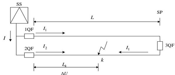
Figure 4: Diagram of double line power supply
