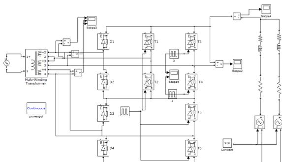
Figure 10: Simulation model of Shaoshan SS4
