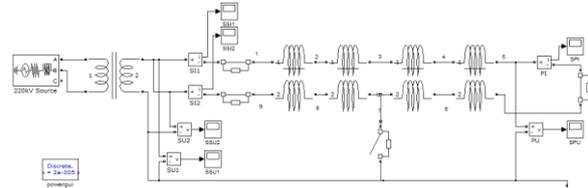
Figure 9: Simulation model of traction power supply system
