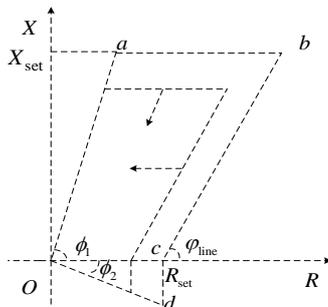
Figure 3: Adaptive distance protection operating characteristic
