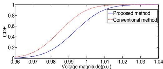
Figure 6: CDF comparison for the magnitude of the voltage at node 34
