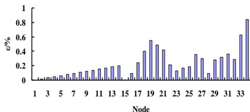
Figure 8: Relative error of the mean value of the magnitude of the node voltage
