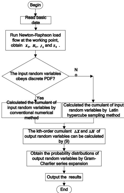
Figure 1: Flow Chart of a PDF Calculation in this work
