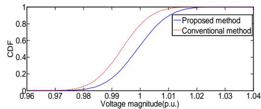
**Figure 5: CDF comparison for the magnitude of the voltage at node 19**
