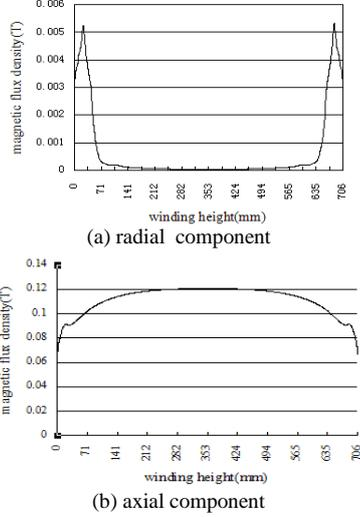
Fig. 6. The distribution of magnetic flux density along LVW inner side height
