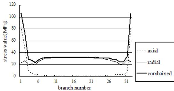
Fig. 7. The distribution of mechanical stress along branches of LVW.
