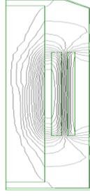
Fig. 5. The leakage magnetic field distribution.
