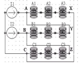
Fig. 2. Equivalent circuit of HVW
