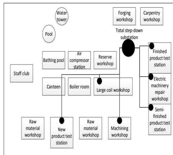
**Figure 3: Location of substations in motor repair plant**
