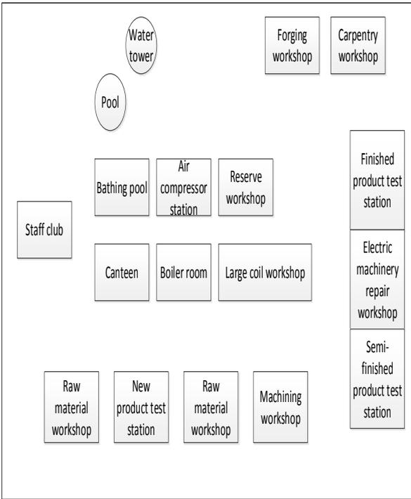
Figure 1: General plan of motor repair plant
