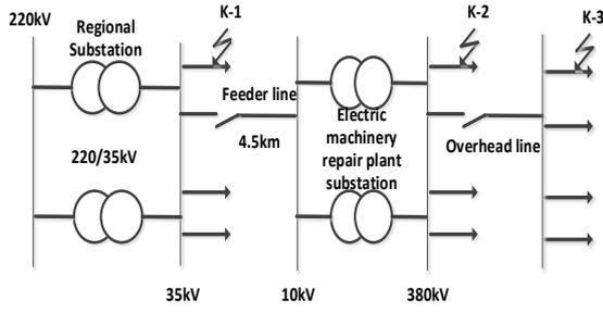
**Figure 5: The equivalent circuit for calculating short circuit current**
