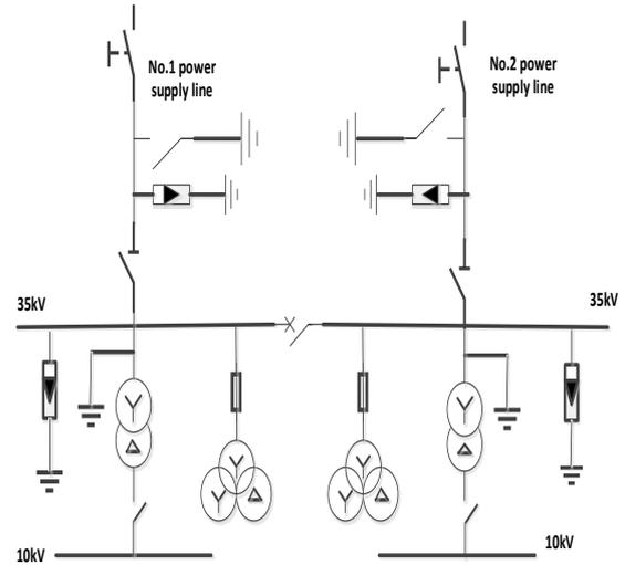
**Figure 4: Main wiring scheme of 35kV total step-down substation**
