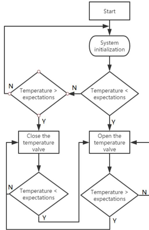
Figure 7 Temperature control flow chart
