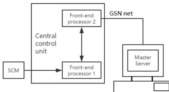
Figure 5 The structure of the data remote communication
