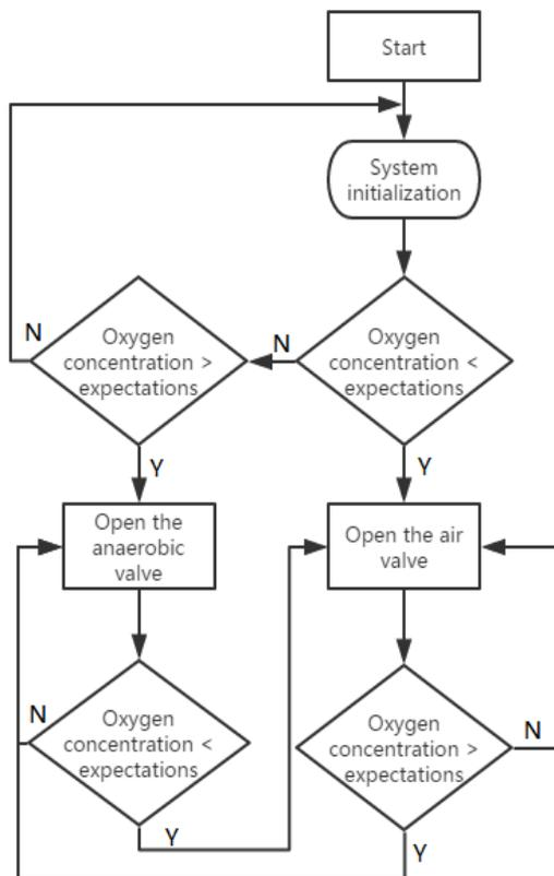
Figure 6 Oxygen concentration control flow chart
