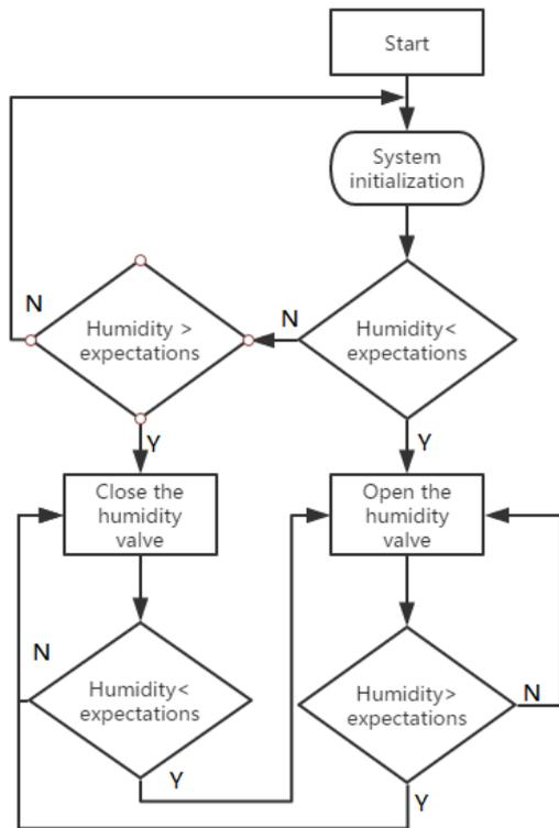
Figure 8 Humidity control flow chart
