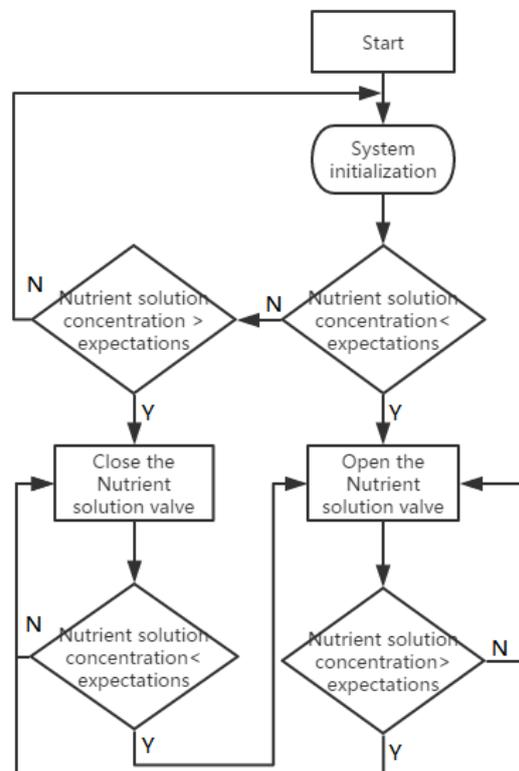
Figure 9 Nutrient concentration control flow chart
