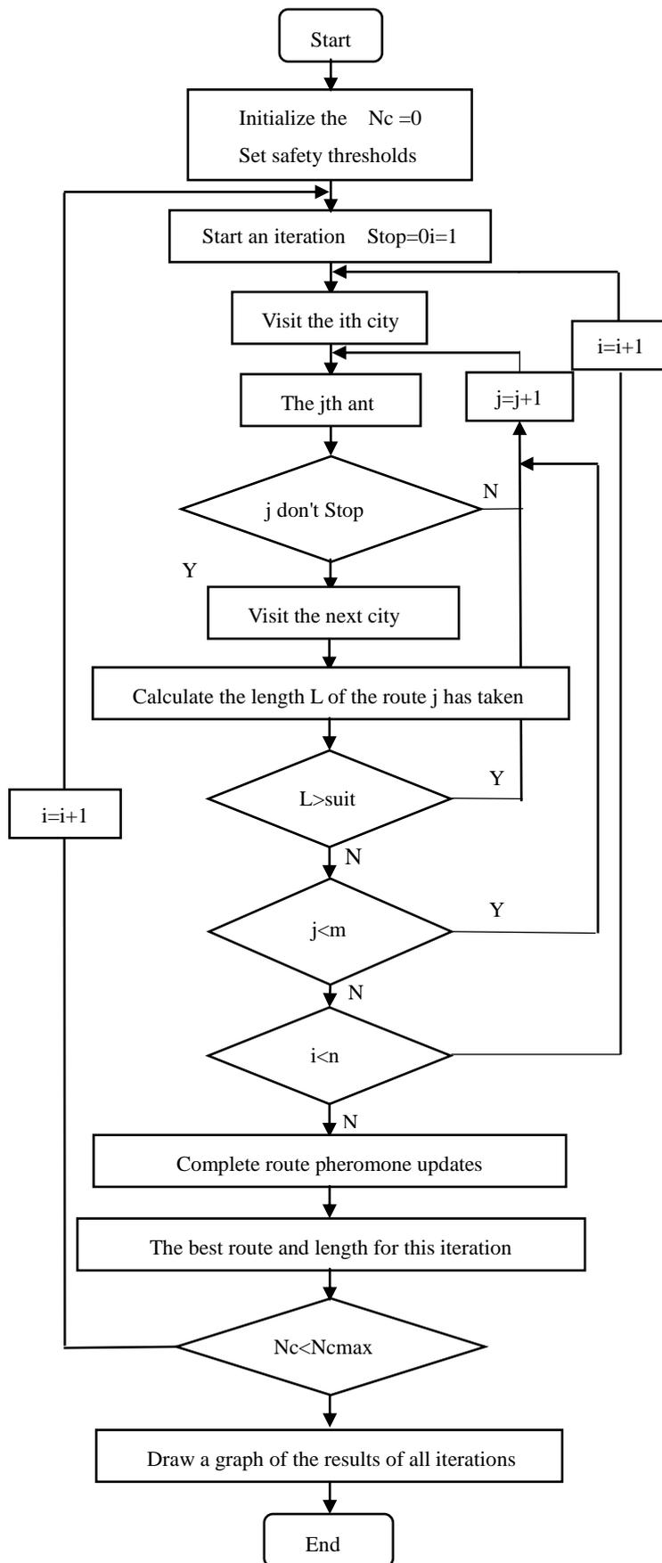
Figure 1 flow chart of improved ant colony algorithm
